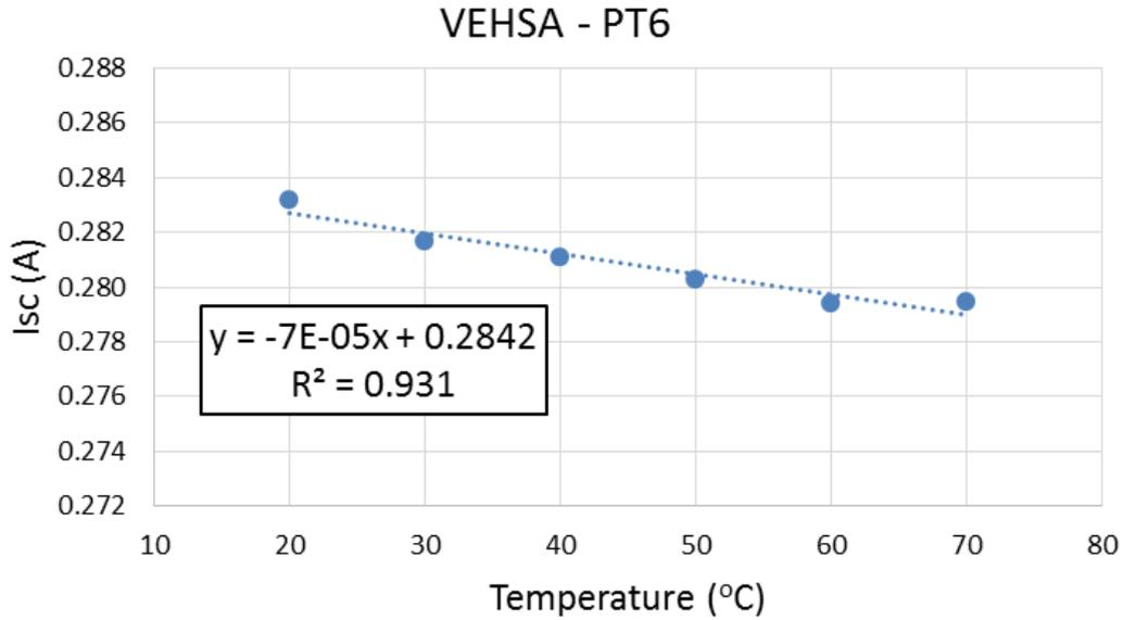
Figure 4. Temperature dependence for a PT6 device measured at 3W optical input, showing the measured short circuit current ( $I_{sc}$ ) dependence.
