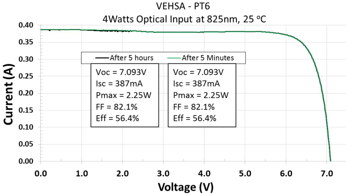
Figure 6. *I-V* data obtained on a new device operated continuously at 4 W of optical input power for 5 minutes compared to 5 hours of continuous operation.
