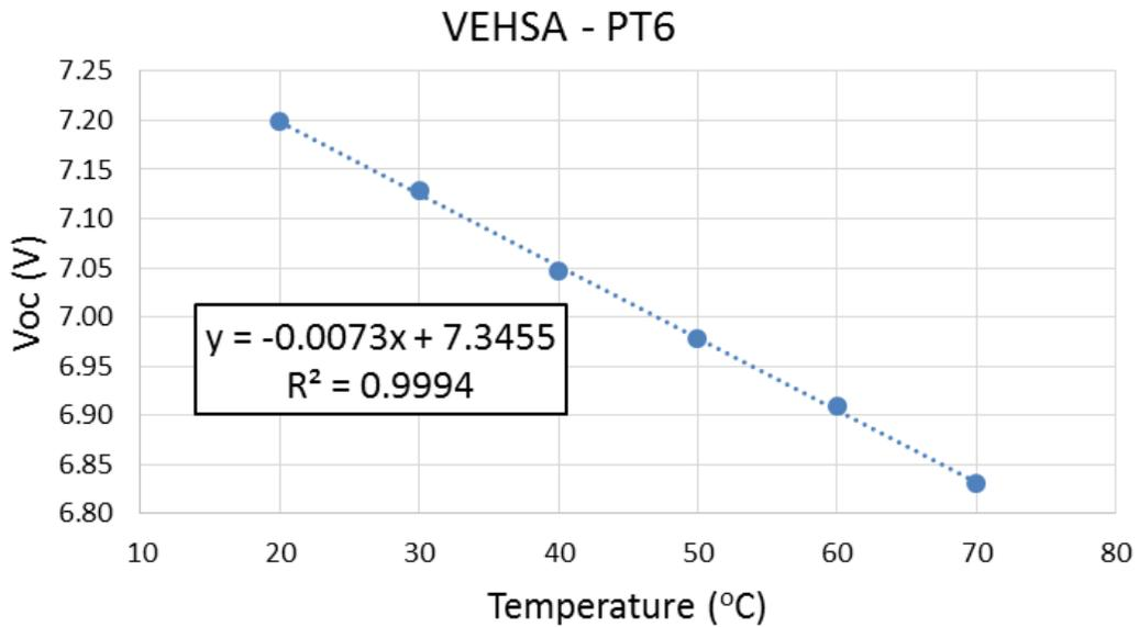
Figure 3. Temperature dependence for a PT6 device measured at 3 W optical input, showing the measured open circuit voltage ( $V_{oc}$ ) dependence.
