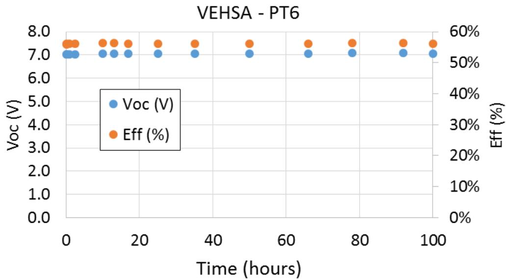
Figure 7. Time dependence of the performance of a PT6 device for 100 hours of continuous operation with an input power of 4 W. The  $V_{oc}$  and the efficiency are unaffected (left and right axes, respectively), similarly the  $I_{sc}$  and the  $FF$  remained constant (not shown) with values as per Figure 6 within about 1% relative and therefore within the experimental error.
