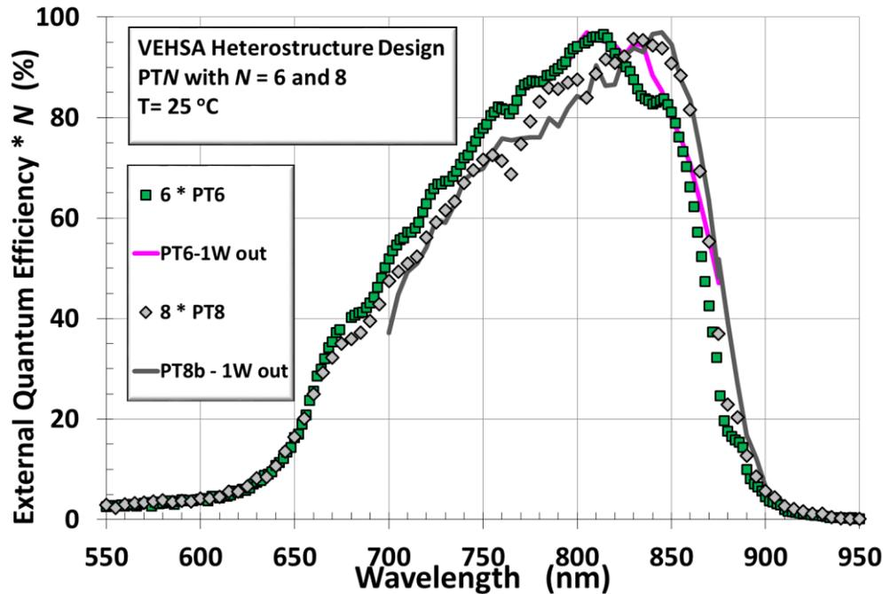
Figure 1. Spectral response of PT6 and PT8 devices. The data with the symbols is obtained at very low power using a standard quantum efficiency (QE) system, whereas the solid lines are measured with greater than 1 W of electrical output with a CW tunable Ti:sapphire laser. The high power measurements have been normalized to obtain the peak value at the same level as the QE data.
