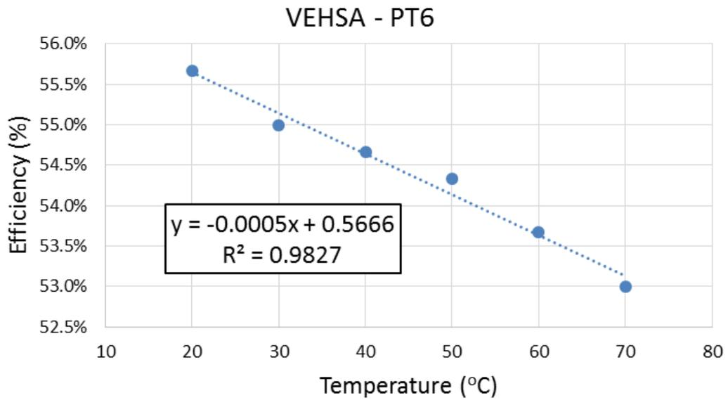
Figure 2. Temperature dependence for a PT6 device measured at 3 W optical input, showing the measured efficiency dependence.
