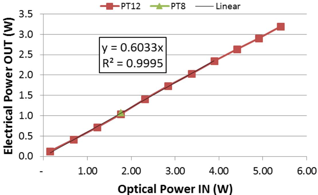
Figure 8. Efficiency measurements for PT8 and PT12 VEHSAs devices excited with a high-power laser diode at 850 nm. The efficiencies are best obtained directly from the slope of the Power IN vs Power OUT linear fit given the strong correlation factor measured. The efficiencies obtained at that wavelength are 60.9% and 60.3% for the PT8 and PT12, respectively. Only one point is displayed for PT8, but it yields very similar measured values as the PT12 device.
