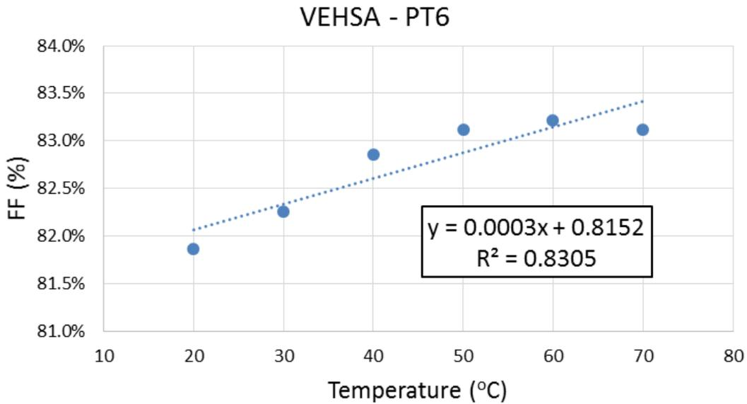
Figure 5. Temperature dependence for a PT6 device measured at 3W optical input, showing the measured fill-factor ( $FF$ ) dependence.
